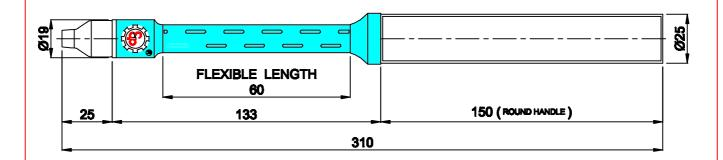
NOTE: 1) ALL DIMENSIONS ARE IN MM 2) HEAD LENGTH WILL VARY AS PER LENGTH OF ARGON ARC NOZZLE
