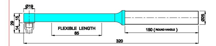
NOTE: 1) ALL DIMENSIONS ARE IN MM 2) HEAD LENGTH WILL VARY AS PER LENGTH OF ARGON ARC NOZZLE
