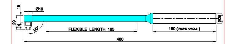
NOTE: 1) ALL DIMENSIONS ARE IN MM 2) HEAD LENGTH WILL VARY AS PER LENGTH OF ARGON ARC NOZZLE
