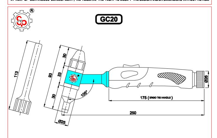
NOTE: 1) ALL DIMENSIONS ARE IN MM 2) HEAD LENGTH WILL VARY AS PER LENGTH OF ARGON ARC NOZZLE
