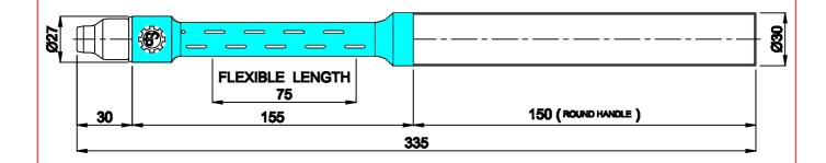
NOTE: 1) ALL DIMENSIONS ARE IN MM 2) HEAD LENGTH WILL VARY AS PER LENGTH OF ARGON ARC NOZZLE
