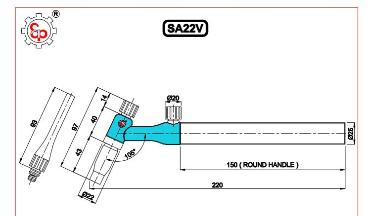
NOTE: 1) ALL DIMENSIONS ARE IN MM 2) HEAD LENGTH WILL VARY AS PER LENGTH OF ARGON ARC NOZZLE
