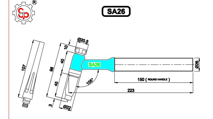
NOTE: 1) ALL DIMENSIONS ARE IN MM. 2) HEAD LENGTH WILL VARY AS PER LENGTH OF ARGON ARC NOZZLE
