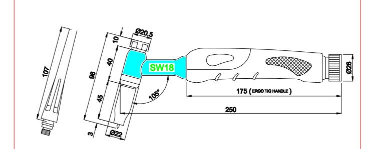
NOTE: 1) ALL DIMENSIONS ARE IN MM. 2) HEAD LENGTH WILL VARY AS PER LENGTH OF ARGON ARC NOZZLE
