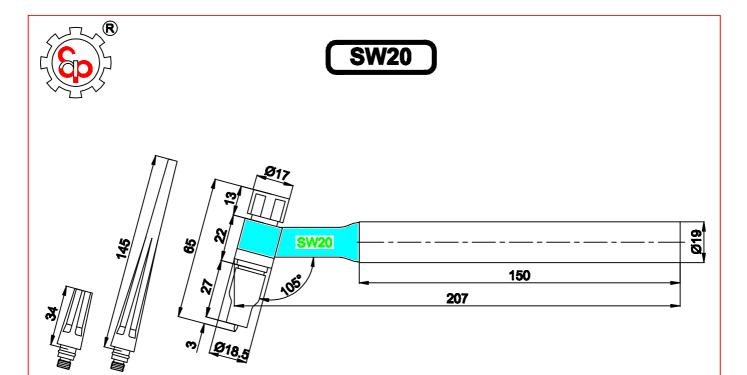
NOTE: 1) ALL DIMENSIONS ARE IN MM. 2) HEAD LENGTH WILL VARY AS PER LENGTH OF ARGON ARC NOZZLE
