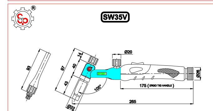
NOTE: 1) ALL DIMENSIONS ARE IN MM. 2) HEAD LENGTH WILL VARY AS PER LENGTH OF ARGON ARC NOZZLE
