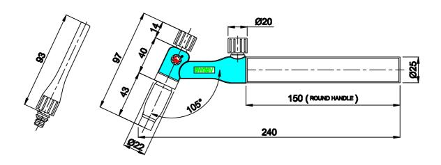
NOTE: 1) ALL DIMENSIONS ARE IN MM. 2) HEAD LENGTH WILL VARY AS PER LENGTH OF ARGON ARC NOZZLE
